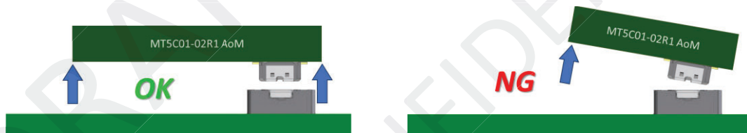
Figure 5-8. Correct Handle when mating a connector
