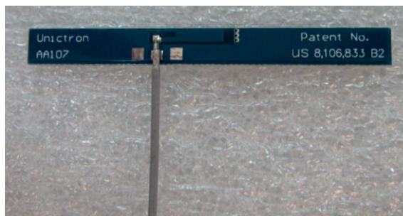
Figure 8-1. 2.4GHz PCB Antenna
